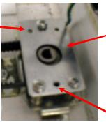
New top X Motor Bracket. Note this bracket does not have a brass collar.
